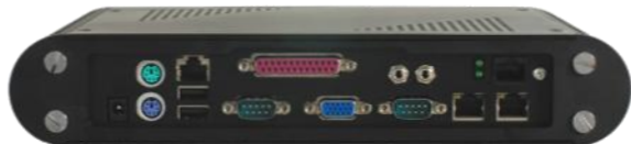
Above: Rear of the Access Controller FB-10 showing various connectivity options.
